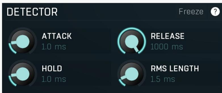
Detector panel contains envelope detector parameters.
