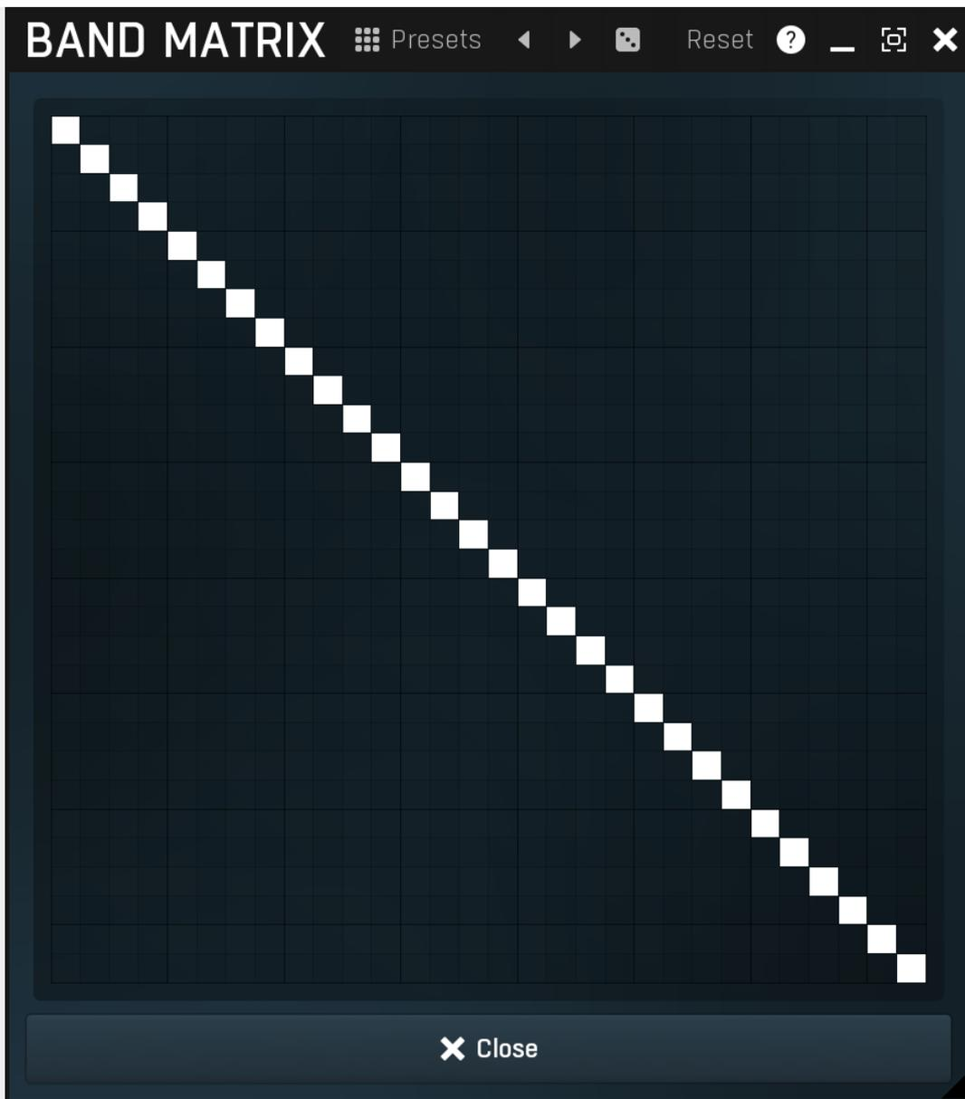
Band matrix controls how the bands affect each other. By default the graph is a diagonal line from top left to bottom right, which means that modulator band 1 affects carrier band 1, modulator band 2 affects carrier band 2 etc. However you may set this up differently and you may even let some carrier bands be affected by multiple modulator bands, or none of them.
