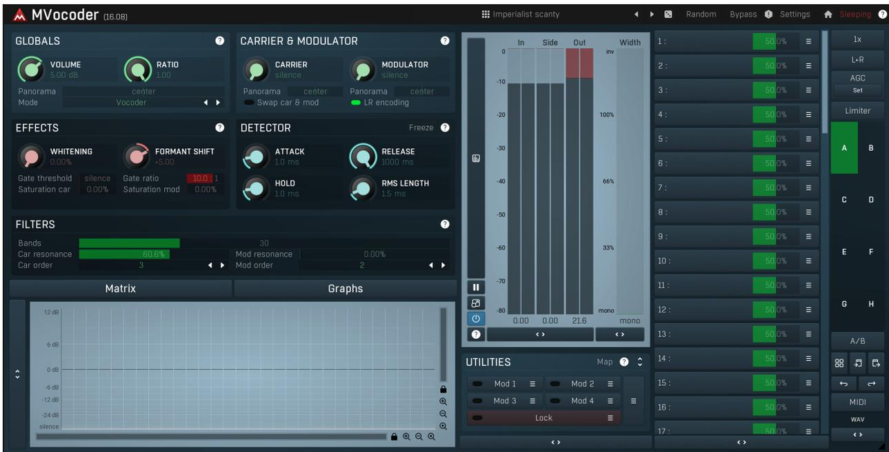
MVocoder is an extremely advanced filter-based vocoder that you can use to generate a robotic voice, make your synth sing etc.
