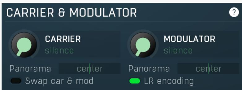
Carrier & modulator panel contains parameters controlling routing and direct carrier & modulator output.
