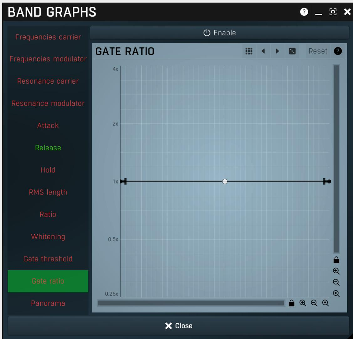
Band graphs window provides a set of graphs, which you can use to control features of each band, such as the distribution of the bands along the frequency axis, resonances, dynamic properties etc.
