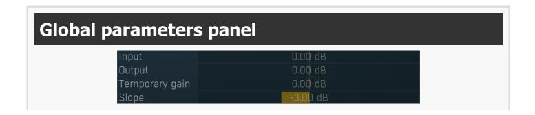
Global parameters panel contains global controls, which are usually relevant to global processing performed either before the signal reaches the crossover and gets split into bands, or after the signals are processed and summed back to the master signal.
