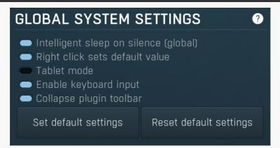
Global system settings panel contains settings which are applied to all plugins on this computer.
