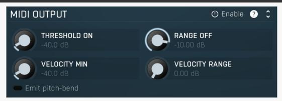
MIDI output panel contains parameters of the integrated audio->MIDI converter. You can use it by accessing the plugin's MIDI output. Please refer to your host's documentation for details about MIDI routing.
