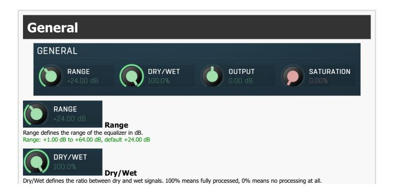
Note that in the case of minimum-phase (not linear-phase) equalizers this is actually not technically possible, without going back in time. So the plugin simulates it by modifying the actual filters where possible. However the low-pass, high-pass, band-pass and notch filters cannot be simulated. These filters are left with 100% dry/wet unless the ratio is set to 0%, in which case the whole processing is bypassed.
