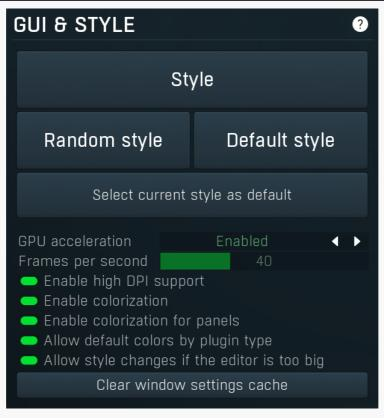
GUI & Style panel lets you configure the plugin's style (and potentially styles of other plugins) and other GUI properties.
