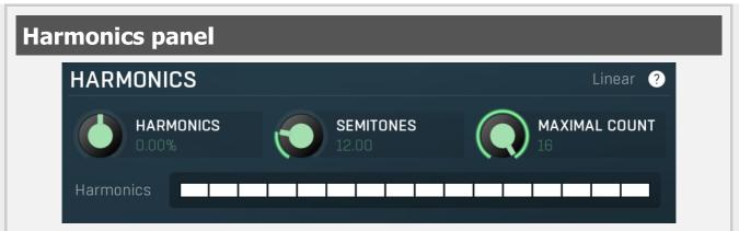
Harmonics panel contains parameters of the harmonics - clones of the main band created at higher frequencies derived from the frequency of the main band. This is often useful for removing natural noises, which usually bring some harmonics with them etc.
