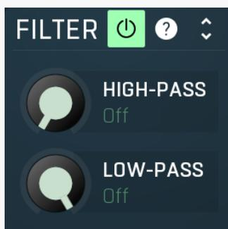
Filter panel contains the HP & LP filters which may be used to compare a specific part of the spectrum.
