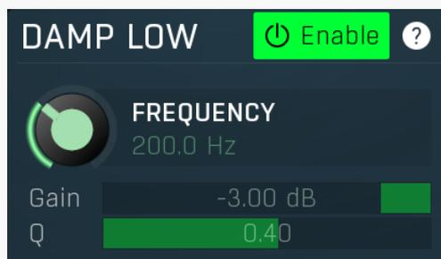
Damp Low panel contains parameters of the low frequency dampening filter. Its purpose is to simulate absorption by air and walls.
