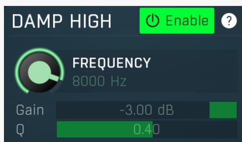
Damp High panel contains parameters of the high frequency dampening filter. Its purpose is to simulate absorption by air and walls.
