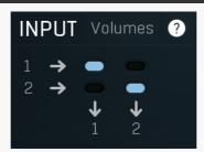
Input channel grid lets you route any input channel into any output channel(s). Left axis shows input channels, bottom axis shows output channels. You can route multiple inputs into a single output, in which case these are mixed together.
