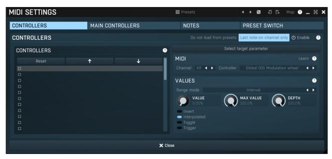
MIDI settings window lets you configure, how the plugin reacts to various MIDI messages. You can use MIDI controllers or MIDI notes and you can also configure a controller to switch between presets, which is especially useful for realtime performances.
