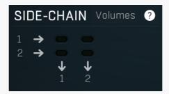
Side-chain channel grid lets you route any side-chain input channel into any output channels. Left axis shows side-chain input channels, bottom axis shows output channels. You can route multiple inputs into a single output, in which case these are mixed together.
