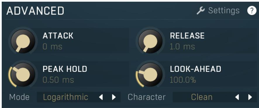
Advanced panel contains more advanced parameters defining how the plug-in determines the level of the source signal, dynamic shape transformation etc.
